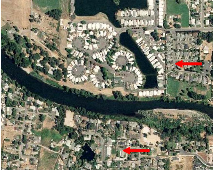
Figure 31-11. The middle mainstem Rogue River is disconnected from its floodplain and wetlands. Red arrows point to disconnected portions. This eliminates stable side channels that provide coho salmon rearing habitat. June 2005.
